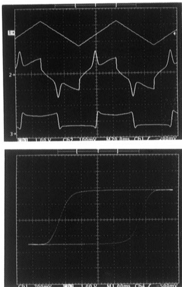
Figure 5. Photographs taken from the oscilloscope; (a, top) The optical and current response (bottom and middle) to a triangular electric field (top) ( 22^\circ ) and (b, bottom) the hysteresis loop used for measuring the spontaneous polarization of A2c in the S_C^* phase ( 26^\circ ).
